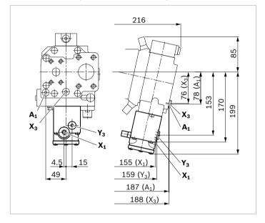
▼ DR/DRG - Pressure controller/pressure controller remotely controlled
