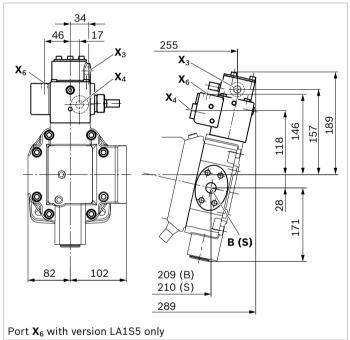
▼ DR/DRG - Pressure controller/pressure controller remotely controlled
