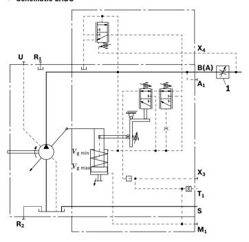
The measuring orifice (control block) (1) is not included in the scope of delivery.
