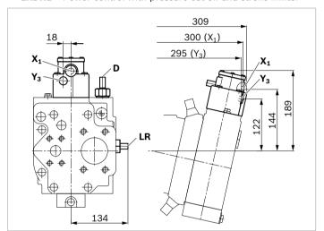
▼ DR/DRG - Pressure controller/pressure controller remotely controlled
