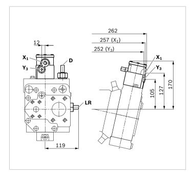
▼ LRDS - Power control with pressure cut-off and load sensing
