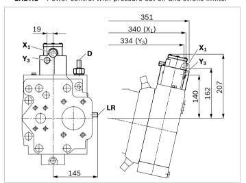
▼ DR/DRG - Pressure controller/pressure controller remotely controlled
