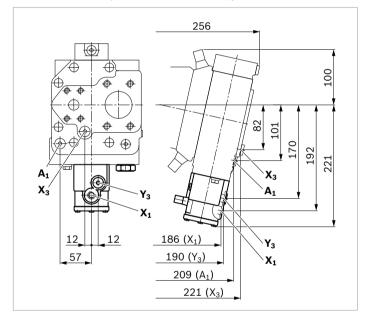
**▼ DRS** – Pressure controller with load sensing
