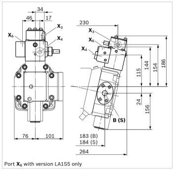
▼ DR/DRG - Pressure controller/pressure controller remotely controlled
