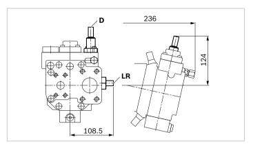
▼ HD1, HD1G - Proportional hydraulic control, positive control, and variant with pressure cut-off, remotely controlled
